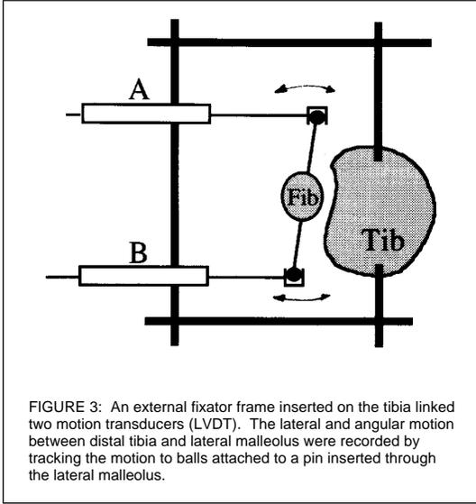
FIGURE 3: An external fixator frame inserted on the tibia linked two motion transducers (LVDT). The lateral and angular motion between distal tibia and lateral malleolus were recorded by tracking the motion to balls attached to a pin inserted through the lateral malleolus.
