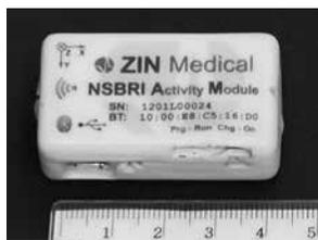
Figure 1: AMU which was attached to the tibia and waist belt.
