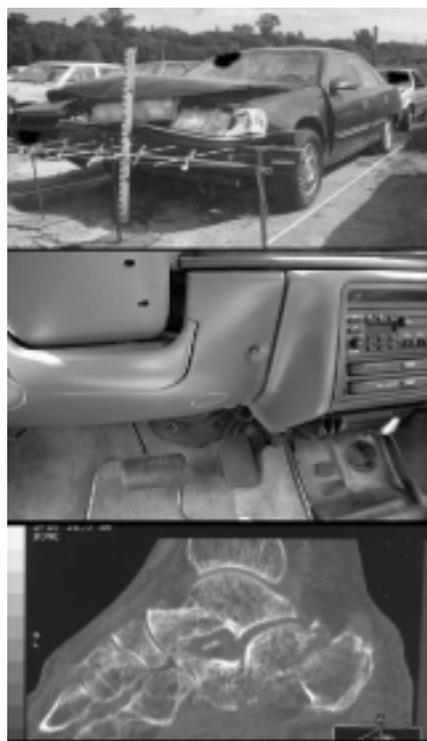
Figure 1: Example crash from CIREN data showing (upper) the frontal collision of the vehicle, (middle) lack of any significant intrusion into the footwell area, (lower) the resulting calcaneus fracture.
