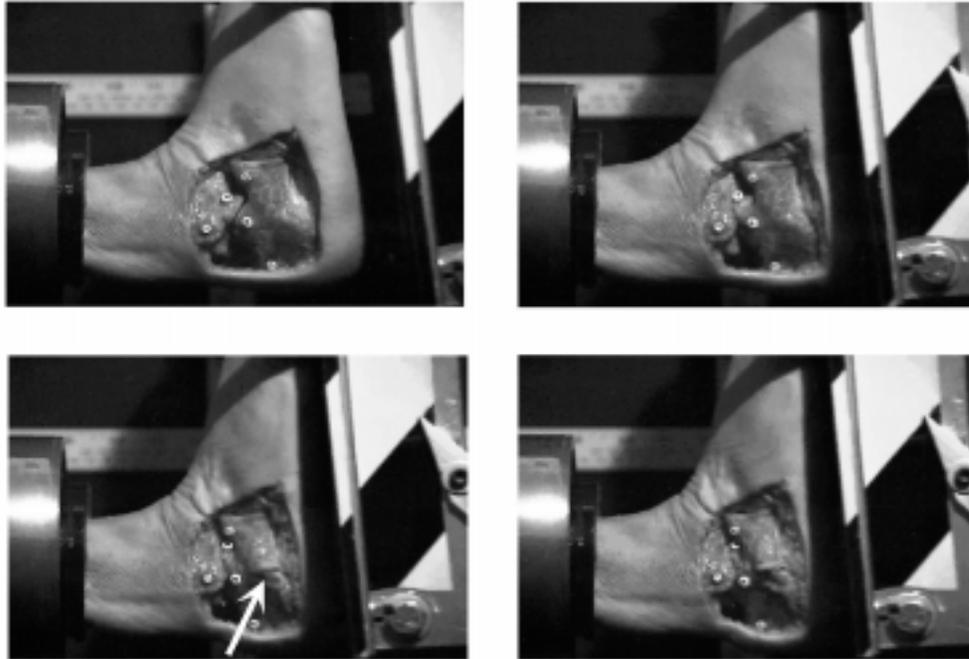
Figure 3: (upper left) dorsiflexed specimen before impact, (upper right) initial contact, (lower left) with loss of joint space crack forms on plantar surface of calcaneus (arrow), (lower right) calcaneus fractured.
