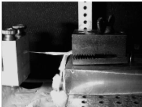
Figure 3: Tensiometric Force Testing of Healing Tendon.
