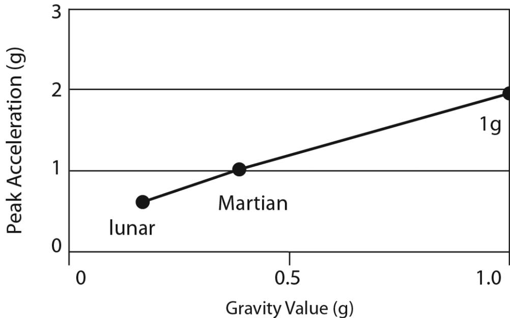
Figure 4: Mean peak tibial acceleration (n=3) during walking at 3 different gravity levels.
